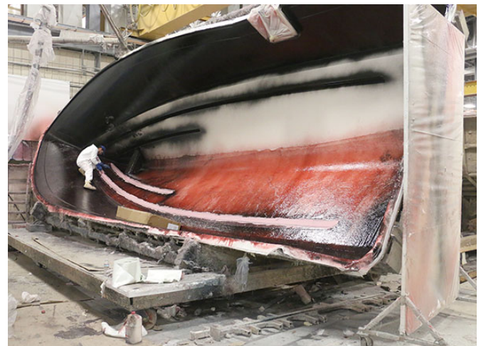
Mold for one of the larger Grady White boats
